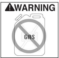
Never use gasoline or other flammable liquids to clean this tool. Vapors in the tool may ignite, causing the tool to explode. Ignoring this warning may lead to serious personal injury or even death!
